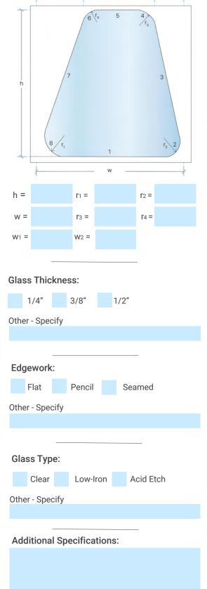
Please mark any fabrication needs, edgework, hole drilling, notching, cut-out, etc.
